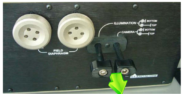
Figure 4.5: Top view optics on Dual View Stand Alone base require illumination and camera shutters to be pulled out.
