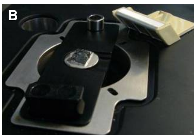
Figure 11.2.7.5: Surface charge can affect cantilever deflection in force-distance curves: A) attractive forces pulling cantilever towards surface in approach; B) Eliminating charge by removing any glass components in sample mounting. Here, the sample (graphite) is fixed to sample puck via silver paint, and placed on an AR magnetic sample holder, and the use of a Static Master.
