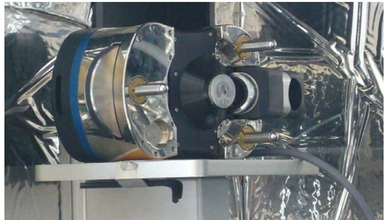
Figure 6.2.8: Place head on its side after use in fluid to allow gravity to remove fluid safely.
