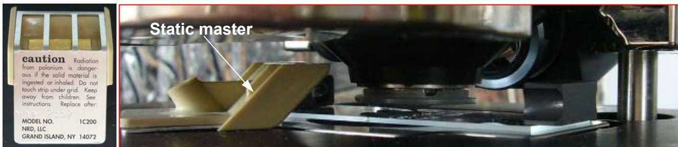
Figure 6.1.13: Placing static master near sample to dissipate charge.
