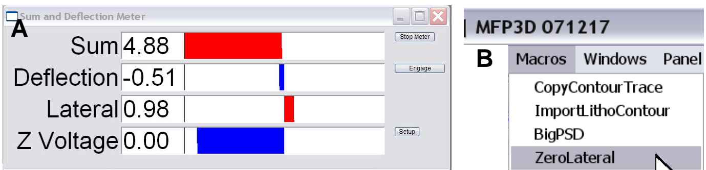
Figure 8.7: Zeroing lateral deflection with LFM Rock ipf: A) typical lateral signal from a given cantilever (see Section 7.7C to view lateral signal): B) with LFM rocks compiled, select ZeroLateral from Macros in menu bar; C) result- electronic zeroing of lateral signal.
