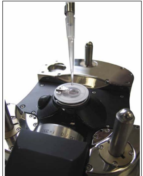
Figure 6.2.1: Wetting the cantilever Photo courtesy of Dr. Irene Revenko
