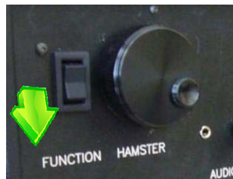
Figure 11.4.1.1: Downward Function toggle to execute force curve when working in Force tab.
