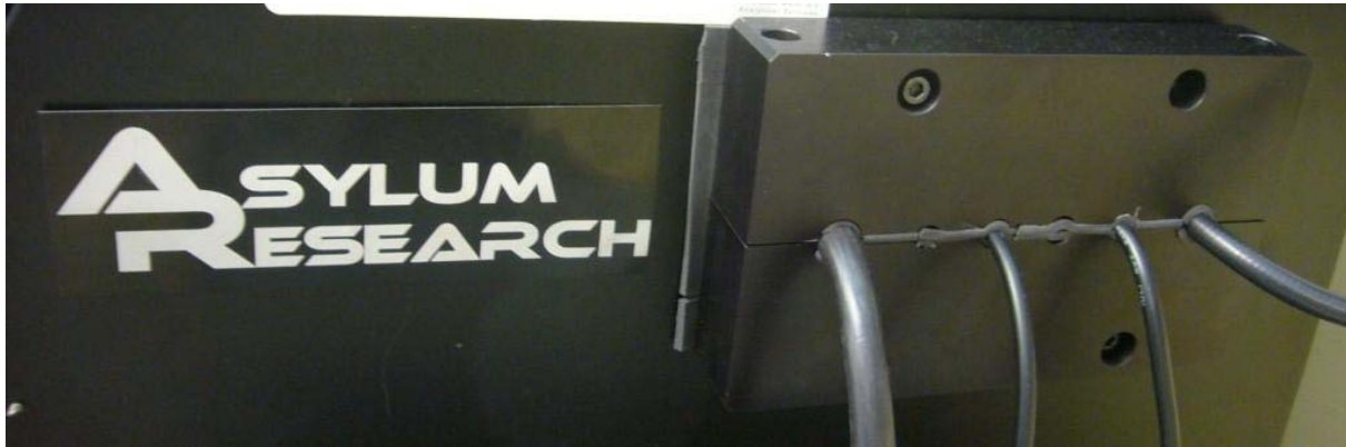
Figure 16.6.2: The cable clamps can offer protection against vibrations traveling down the monster cable, and seal up the acoustic enclosure.
