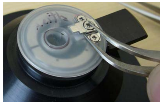
Figure 3.2: GENTLY lifting tongue clamp to accommodate thicker probe chips.
