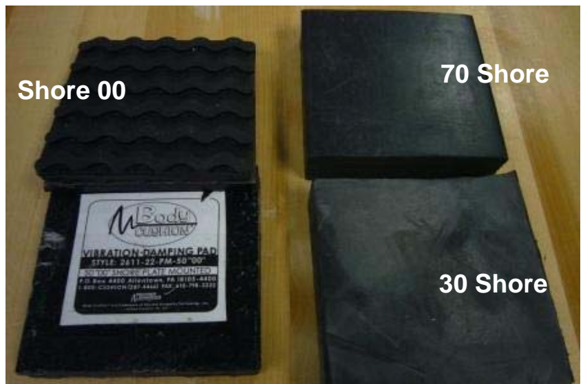
Figure 16.8.1: Different rubber pads used to quell floor vibration coupling into the MFP3D.
